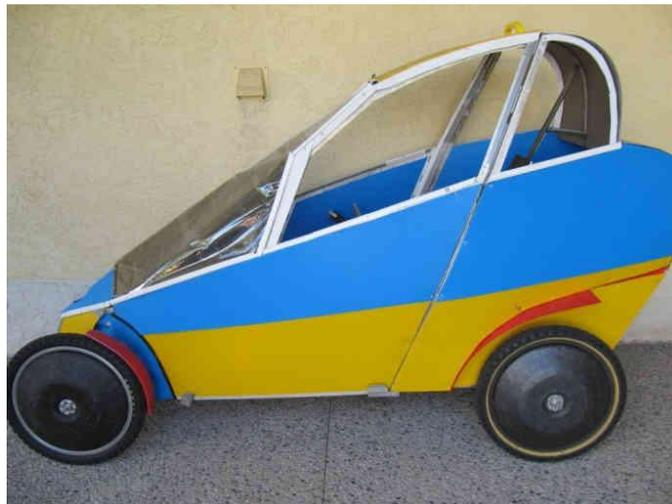
Figure 1 -- Coupe style body with roll-down side windows
