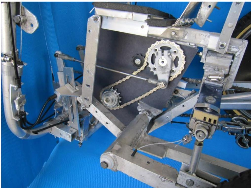
Figure 4 -- Under the seat drivetrain and tilt control elements
