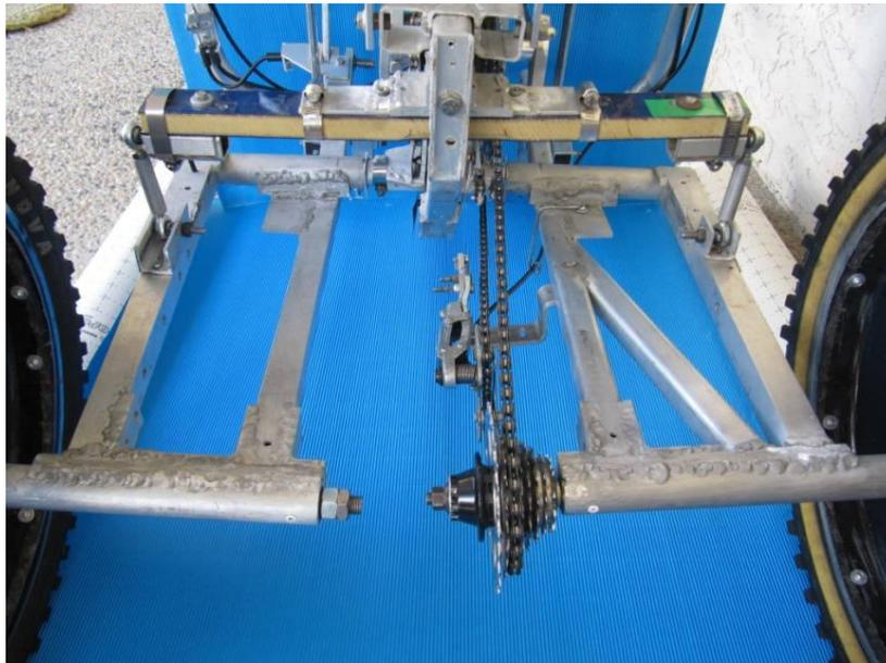
Figure 8 -- Rear swingarms with section of a downhill ski for suspension
