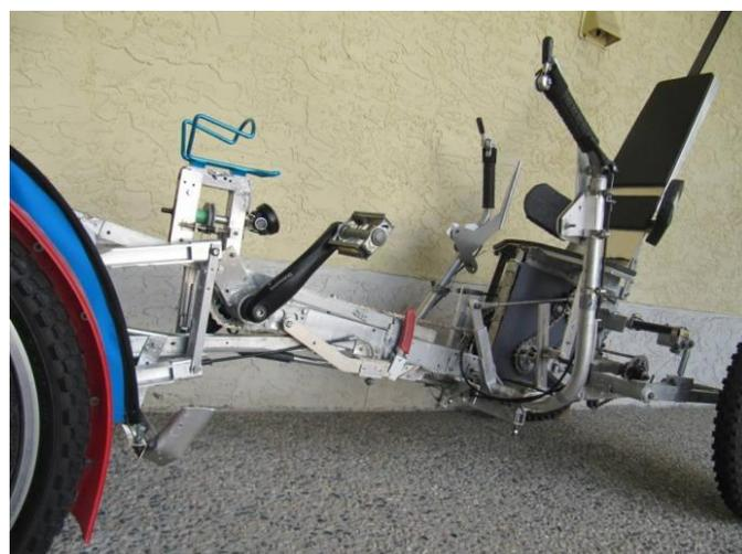
Figure 2 -- Vehicle frame with recumbent seat and arm cranking levers
