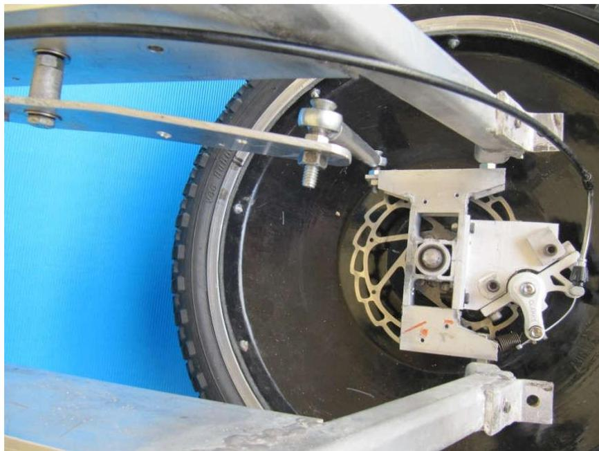
Figure 7 -- Hub, tie rod, and pivot blade beneath swingarm
