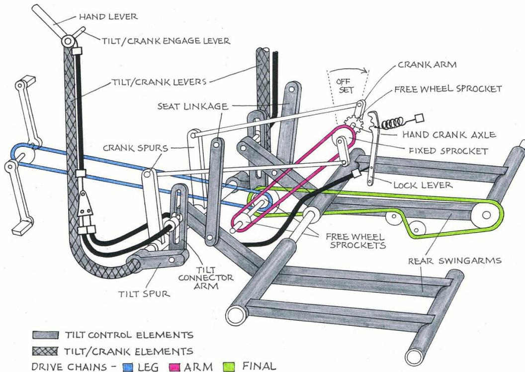
Figure 3 -- Schematic of dual drive system and tilt control elements
