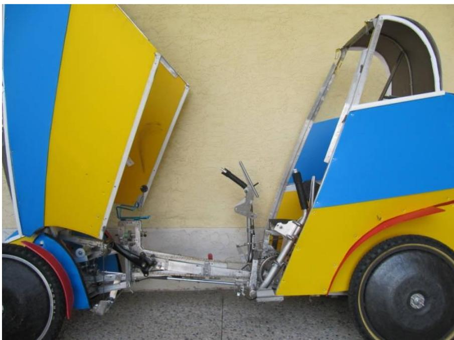
Figure 5 -- Clam door opening for entry/exit
