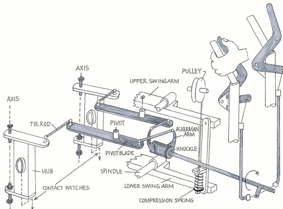
Figure 6 -- Schematic of steering systems
