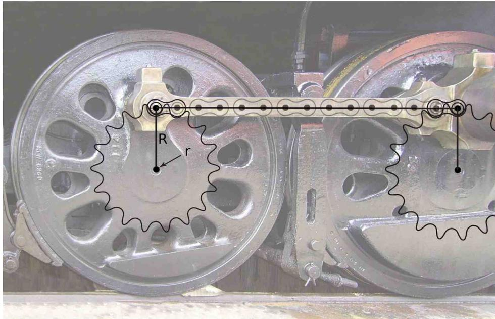
*Figure 2: At the top two joints left and right, a chain between two sprockets is physically equivalent to the connecting rod of a locomotive at  $90^\circ$  from dead center. Background based on photo by Didier Duforest CC-BY-SA 4.0. (The analogy isn't perfect here, as the side rod appears a half-link short.)*
