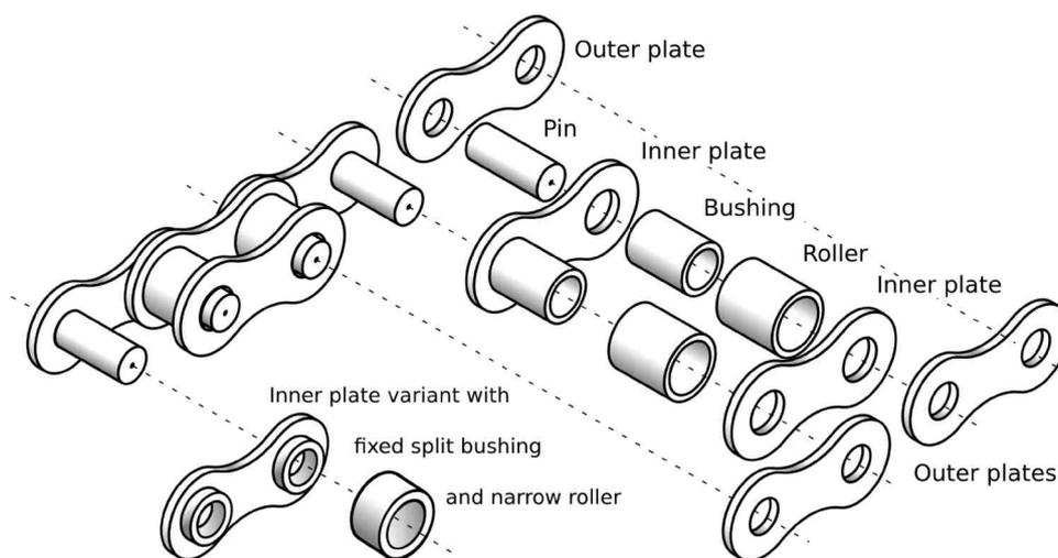
*Figure 1: Roller-chain components, including a modern design for thin chains with one-piece inner plates and half-bushings. Adapted from a drawing by Markus Roeder.*
