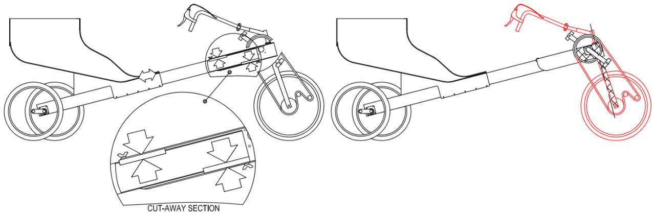
**Figure 15: Leaning trike with separating aluminium frame.**
