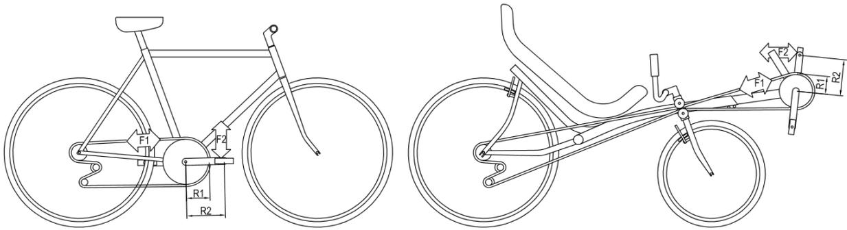
**Figure 2: Chain and leg forces in safety and rear wheel drive recumbent bicycles. In each case, the crank torque is  $F2 * R2$  (Leg) which is the same as  $F1 * R1$  (Chain), so  $F2 = F1 * (R1/R2)$**
