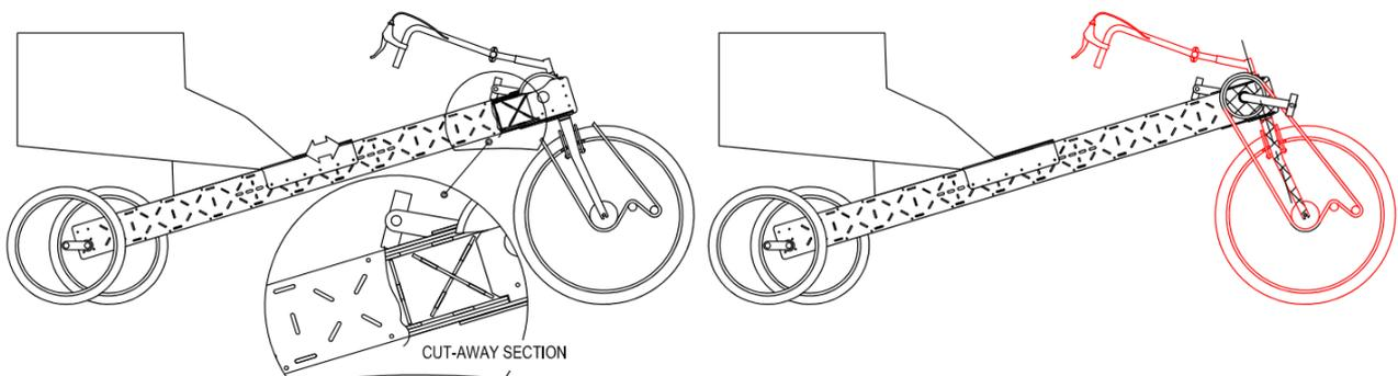
**Figure 16: Leaning trike with plywood frame.**
