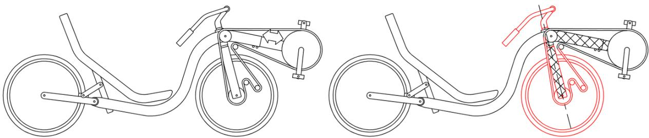
**Figure 7: Toxy front wheel drive bicycle.**
