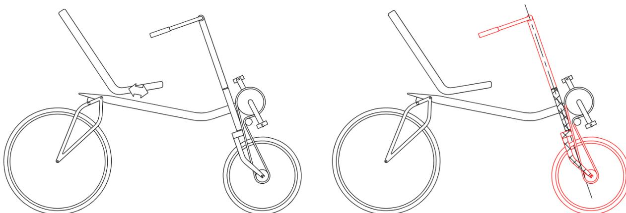
**Figure 11: Bevo front wheel drive bicycle.**
