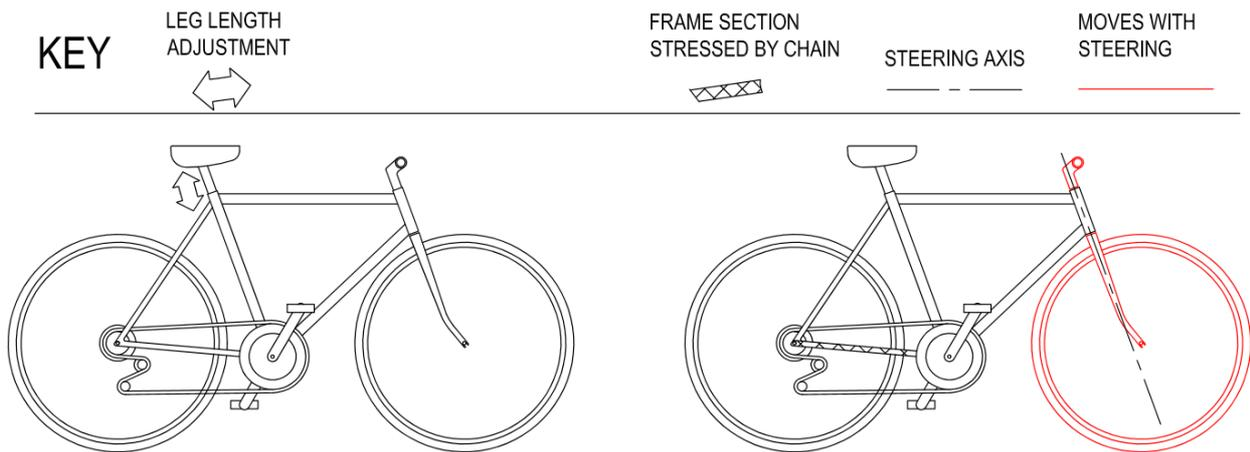
**Figure 3: Safety bike and key to diagrams.**
