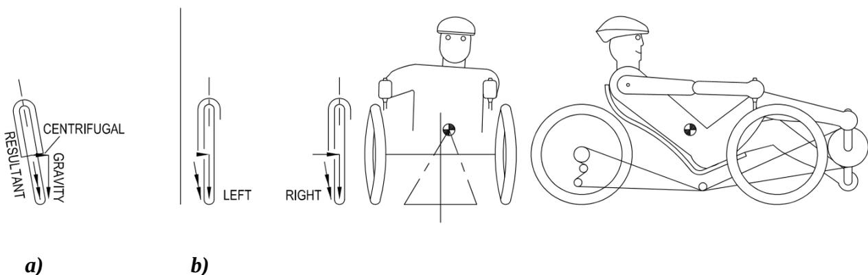
**Figure 1: Leaning dynamics of a) Bicycle / Leaning Trike Wheel which absorbs axial force and b) Standard recumbent trike wheel which must cope with axial force.**
