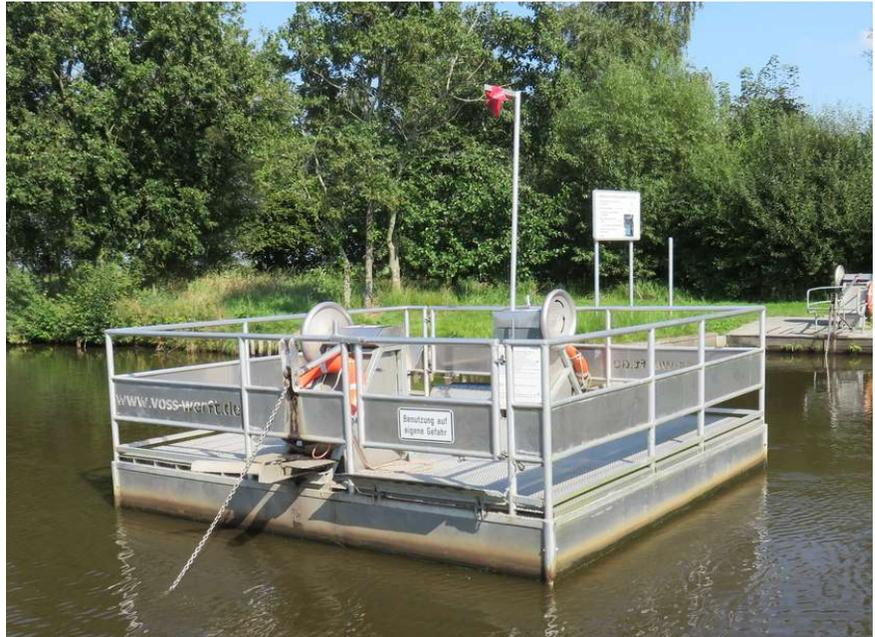
The four self-operated [Lippe-Ferries](#) are available seasonally for 2-8 persons. The chains are operated by crankless flywheels, on the ferry or from the shore. In addition, each has a guidance wire, and one of them a longitudinal rope in order to utilize the current.
