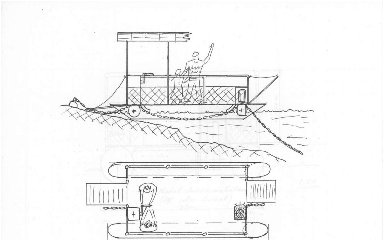
*Example of a simple human-powered chain ferry with a single central chain.*
