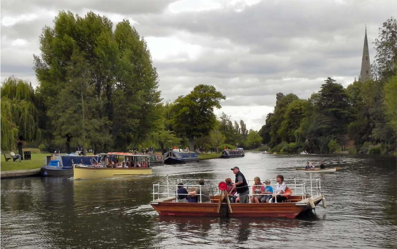
*The chain ferry over the river Avon (GB) is cranked by hand on one side. It is sufficiently slow for the boat on the left to pass safely.*
