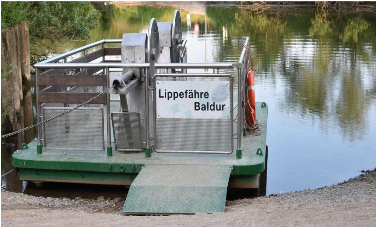
*The [Baldur](#) is one of four [Lippeferries](#) which can transport 2-8 persons "do-it-yourself" over the Lippe in Germany, using flywheels rather than cranks. Besides the one drive chain, the ferries have an additional wire rope for extra guidance.*
