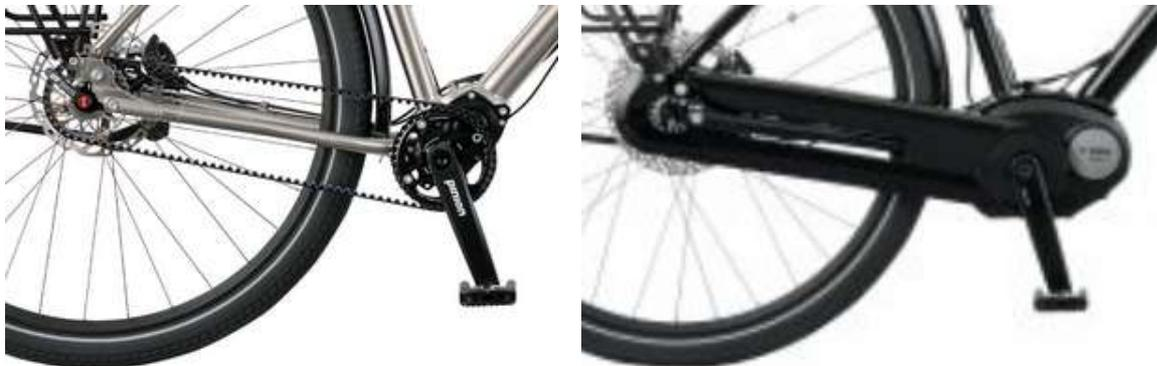
Pinions require special frames, but these types of frames are becoming accepted through the socio-technical frame of ebikes. Electric assist units from Bosch and Shimano have Pinion-like mounting arrangements, so it is possible suppliers making some types of ebikes could consider adapting frames to suit Pinion gearboxes a small step. Several bike reviews (cyclingabout 2018 , dirtmag 2017) point out that Pinion gearboxes resemble electric motors.
