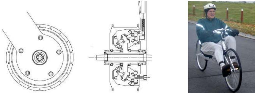
In 2017 Kervelo founder Marc Le Borgne used a new configuration of the Pinion spur gearbox to make and sell a range of front wheel drive recumbent cycles, bringing to life the modular “one direct drive hub, many bicycles” proposal by Kretschmer (2000) through ebike, bicycle, load trike, and leaning trike designs. This adaptation mounted the Pinion gearbox on the bike’s front fork and the front wheel on the Pinion output sprocket.
