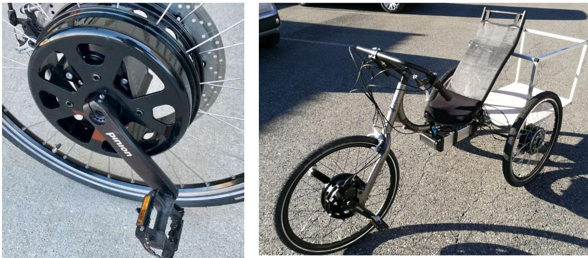
In 2018 Kervelo introduced in-house-built planetary gearboxes with up to 12 gears and a 545% ratio for mounting in front hubs of recumbents and frames of bicycles. Kervelo plan to introduce integrated electric assist for their frame-mounted bicycle gearboxes. Their developments have taken place in parallel, designing fit-for-purpose gearboxes, and simultaneously selling and testing reactions to front wheel drive cycles.
