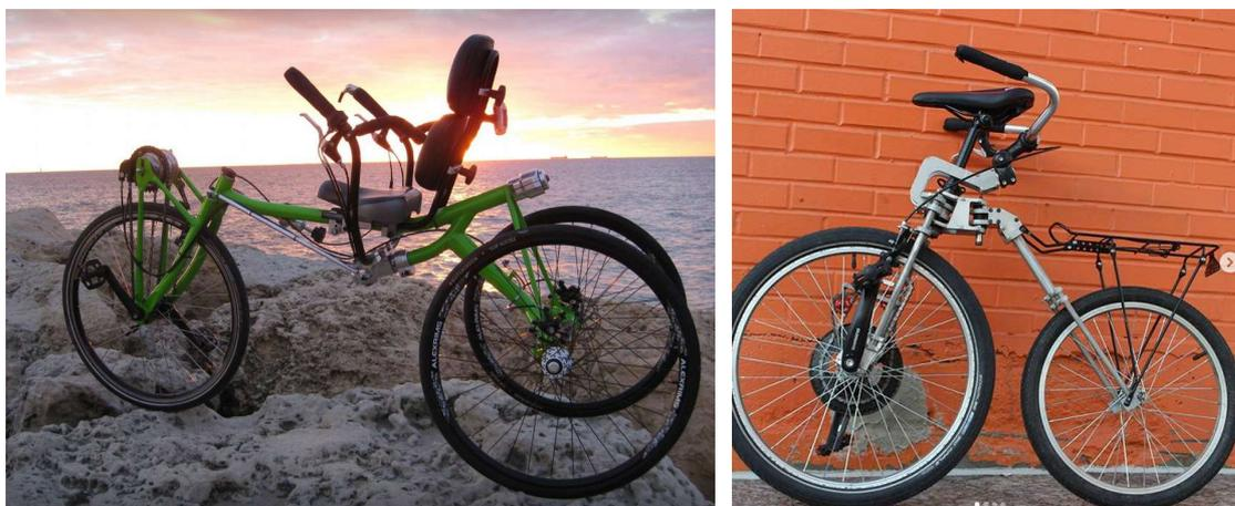
Others including Jeremy Garnet and Marc Le Borgne and have taken up the challenge of producing effective cycles without a chain by developing mechanical gearboxes, and MC2 are producing modular (Fig. 7) versions of
