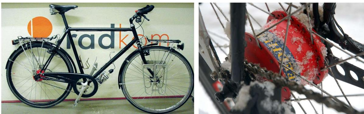
Although the hub's positives were recognized, for some mountain bikers, the Rohloff had issues. It puts weight in the centre of the rear wheel contributing significantly to unsprung mass, causing problems with fully suspended bikes.
