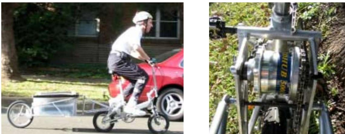
The desirability of the Lahar showed that mountain bike technology could be improved fundamentally, that is by development of a purpose designed, frame mounted, wide ratio gearbox. Pinion Gearboxes fill this niche.
