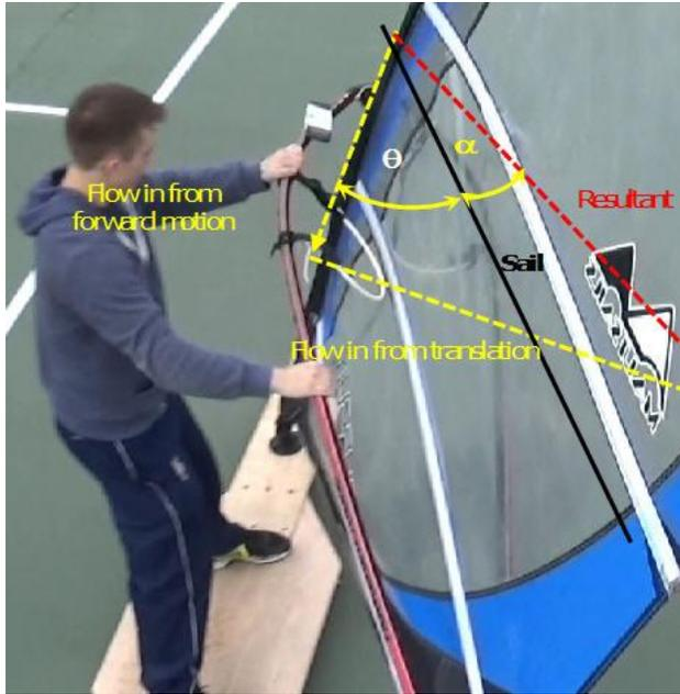
Figure 3. Sail angle of attack and pitch.
