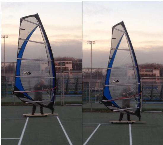
Figure 1. Windsurfer cart under sail pumping power. In the photo at right one can see the sail twists at its aft upper end due to the stroking motion away from the pilot.
