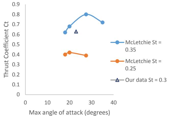
Figure 12. Thrust coefficients for oscillating foils for our results and McLetchie.
