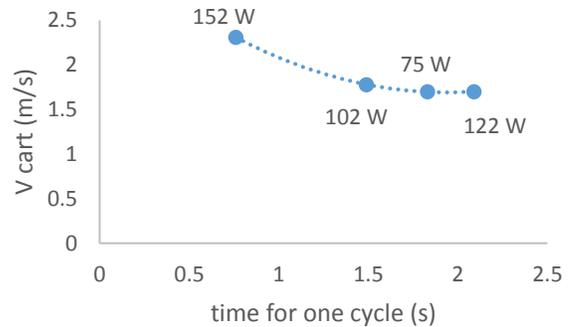
Figure 13. Wattage expended as a function of stroking speed and cart velocity.
