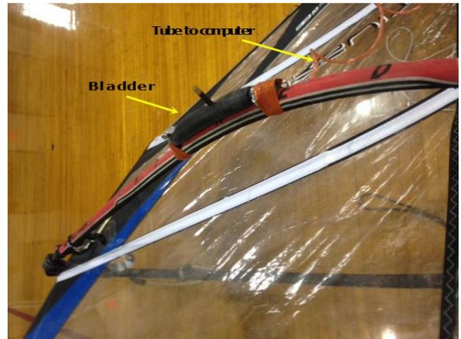
Figure 5. Bladder for measuring force applied by pilot. Bladder is attached to the boom. In this configuration the pilot would push on the bladder as he strokes. For measuring the pulling force the bladder would be rotated around the boom 180 degrees.
