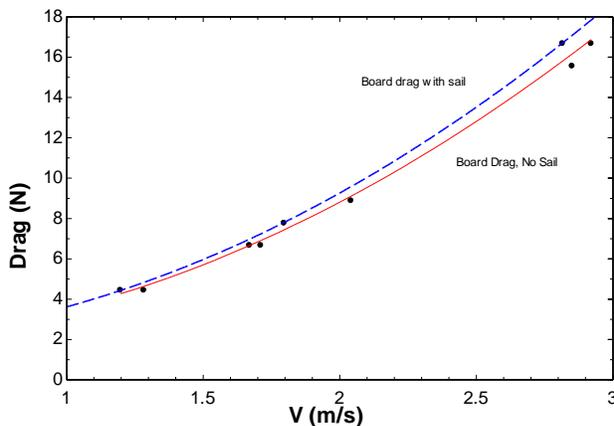
Figure 4. Drag force on rolling board with and without sail rig.
