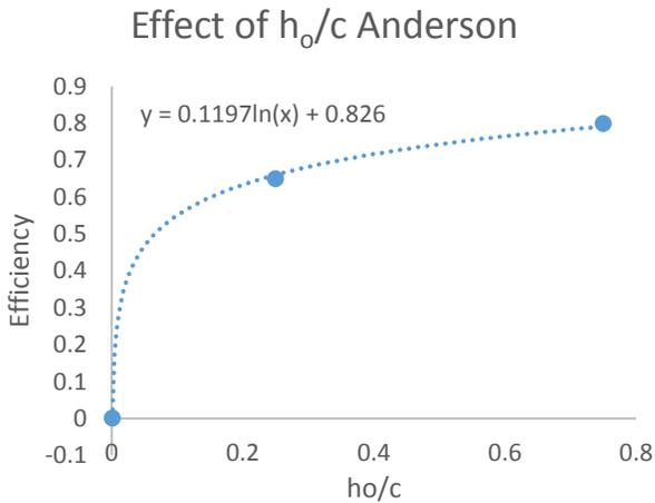
Figure 11. Effect of  $h_o/c$  on efficiency, per Anderson for oscillating rigid foils.
