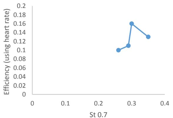
Figure 10. Peak in the efficiency at  $St = 0.3$ .
