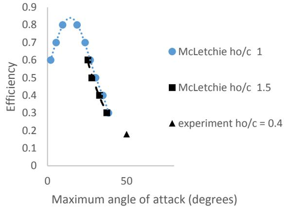
Figure 9. McLetchie's flapping foil data show that efficiency is compromised at higher maximum angles of attack. Our results are shown by the triangle.
