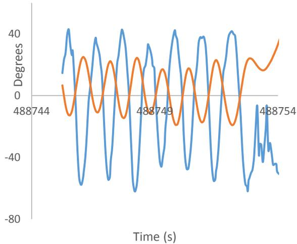
Figure 8. Angle of attack (blue) 2 m over deck (Center of Effort).
