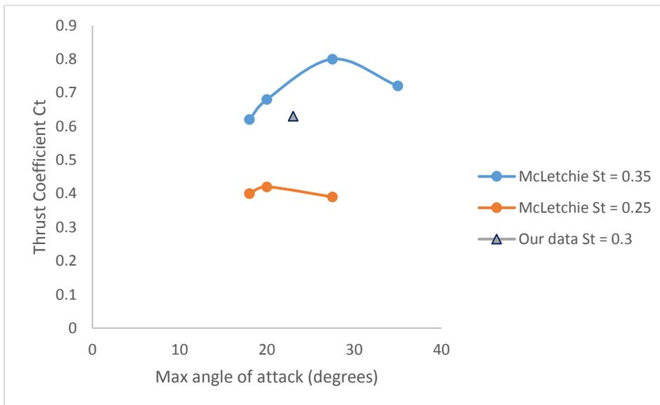
Figure 12. Thrust coefficients for oscillating foils for our results and McLetchie.
