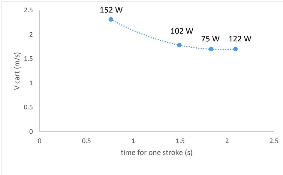
Figure 13. Wattage expended as a function of stroking speed and cart velocity.
