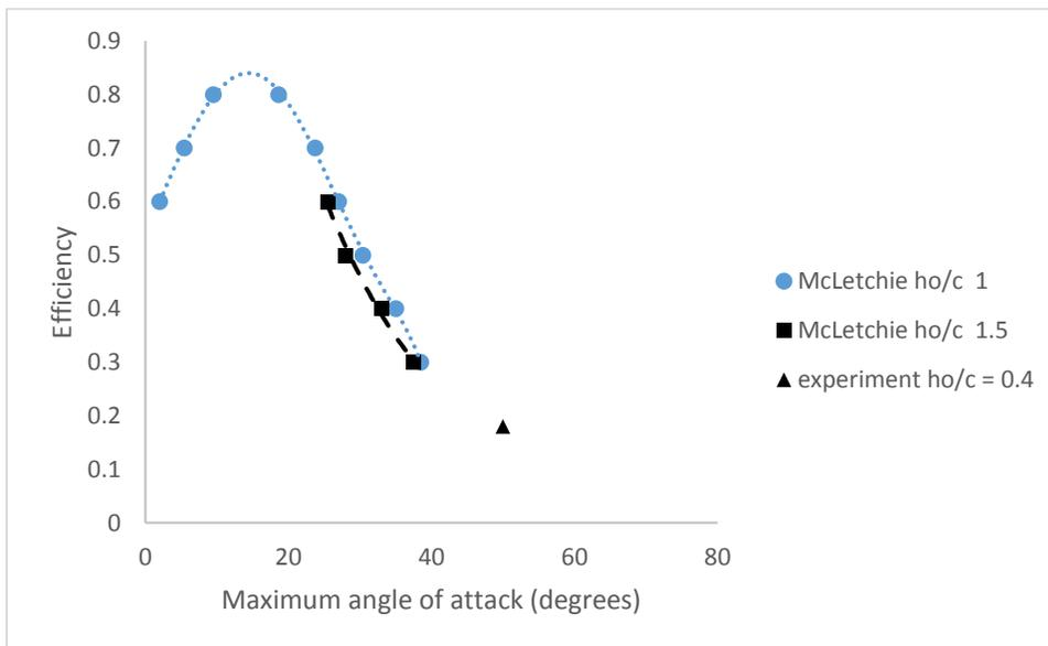
Figure 9. McLetchie's flapping foil data show that efficiency is compromised at higher maximum angles of attack. Our results are shown by the triangle.
