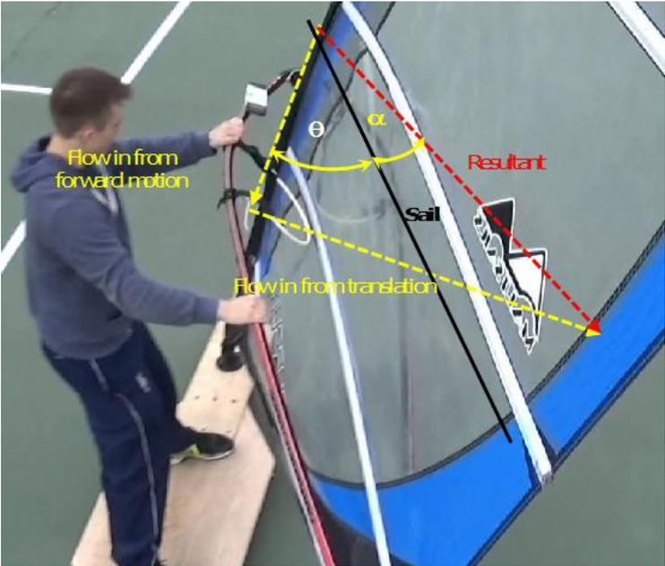
Figure 3. Sail angle of attack and pitch.
