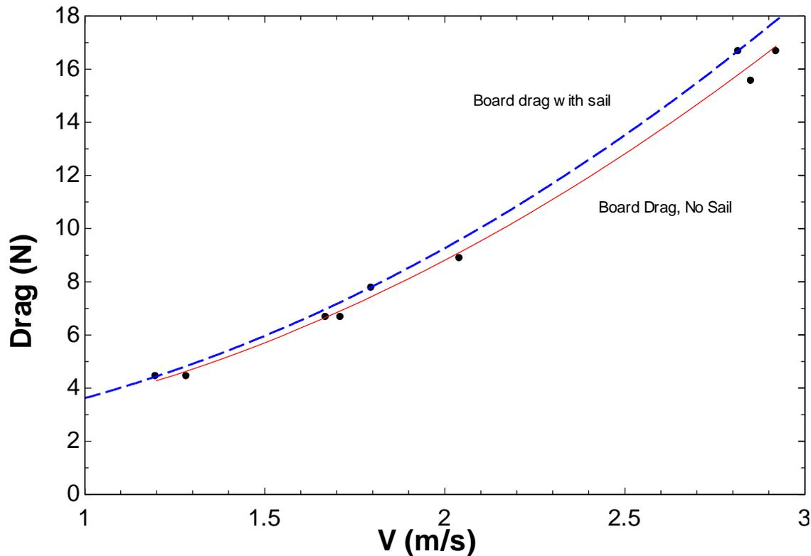
Figure 4. Drag force on rolling board with and without sail rig.
