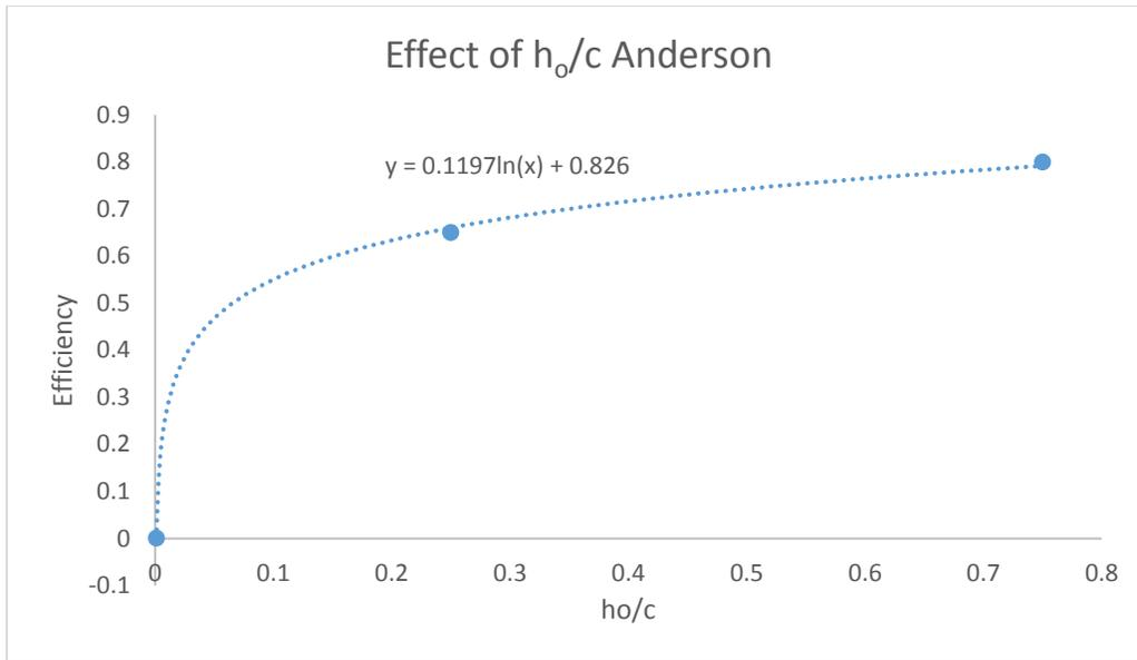
Figure 11. Effect of  $h_o/c$  on efficiency, per Anderson for oscillating rigid foils.
