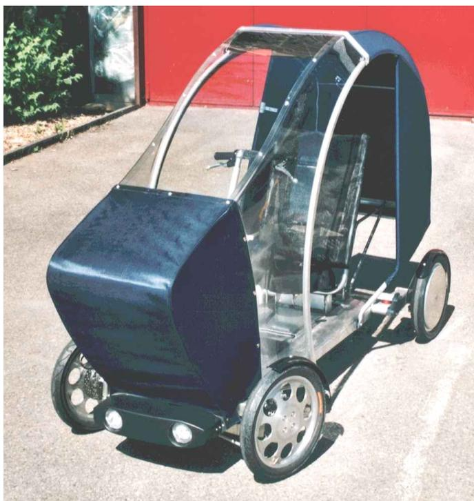
Fig. 2b. Urban Quadracycle prototype, with fairing put onto chassis. Doors foreseen, but not in picture.
