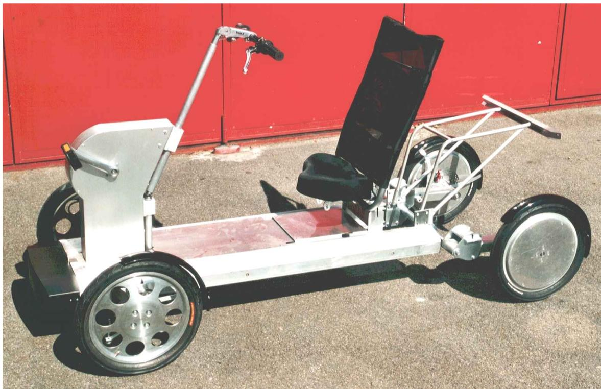
Fig. 2a. Urban Quadracycle, prototype chassis
