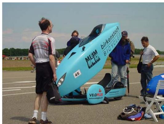
Figure 1: This magnificent tricycle of Jürg Birkenstock has a so-called 'NACA submerged duct' for ventilation. On the photograph the duct is the dark triangle in front of the window. This placement of the intake ensures that the ventilation air is aimed directly at the rider. Not visible on the photograph are two additional air intakes at the underside of the front of the vehicle (photograph courtesy of Robert Biesemans, 2001.)
